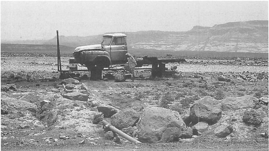
Pumping groundwater near Thula for irrigation, with the help of an Isuzu engine.
